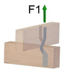
2 Purlin Anchor twist 280 pr. connection
