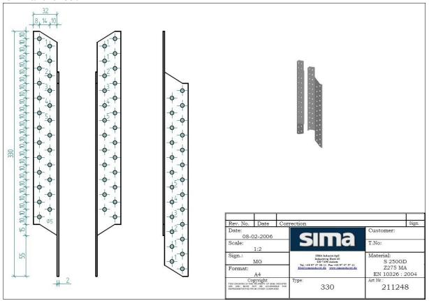
Additionally the bracket can be made from 1,5 mm pre-galvanized steel grades S350GD to Grade S500GD  $\pm$  min. Z275 according to EN 10346 named Purlin Anchor 330PL
