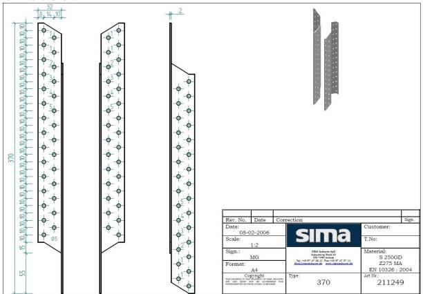
Additionally the bracket can be made from 1,5 mm pre-galvanized steel grades S350GD to Grade S500GD  $\pm$  min. Z275 according to EN 10346 named Purlin Anchor 370PL
