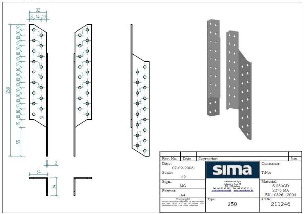
Additionally the bracket can be made from 1.5 mm pre-galvanized steel grades S350GD to Grade S500GD + min. Z275 according to EN 10346 named Purlin Anchor 250PL
